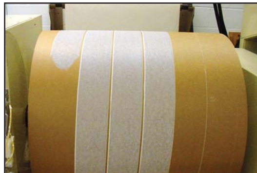
Sheet coated using a CLC-6000™ cylindrical laboratory coater at WMU. Sample will be cut down into sheets that will be dropped into the gravure or flexo press.
